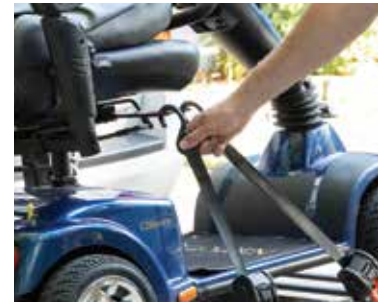
Securement device specialized to type of mobility device.
